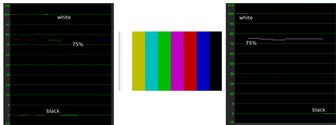
Figure 10.76: Colortest 75% with Waveform RGB (left) and Waveform (right)
